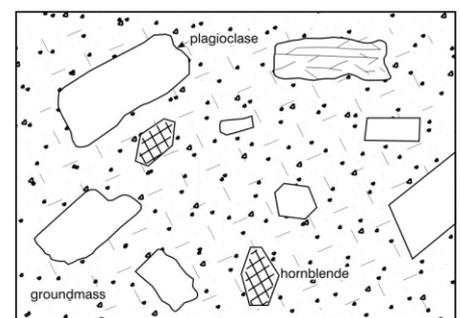
**Figure 4** - View of a porphyritic Andesite under a microscope.
