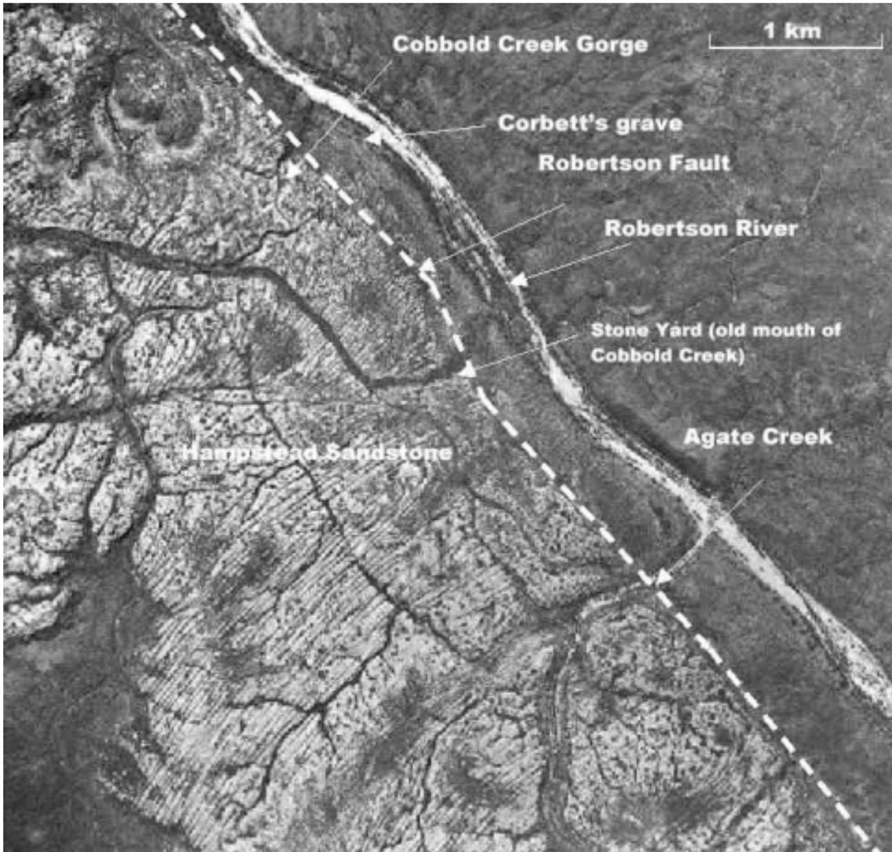
**Aerial photograph of the Cobbold Creek area, showing the white Hampstead Sandstone. The arrays of thin dark lines are prominent joints in the sandstone. The former course of Cobbold Creek, prior to the formation of Cobbold Gorge, can be clearly seen joining the Robertson River near Stone Yard. The dotted line outline the trace of the Robertson Fault. Portion of North Head Run 9 photo 4305, flown 14-5-1972 for the Commonwealth of Australia (used with permission)**
